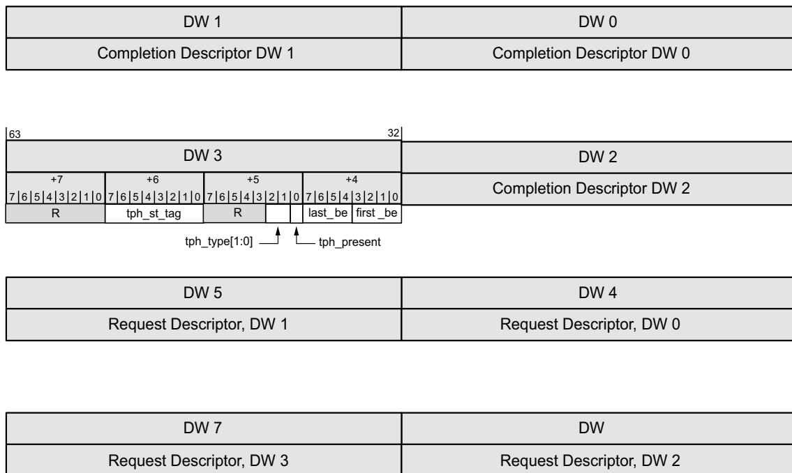
Figure 3-35: Composition of the AXI4-Stream Packet for UR and CA Completions
