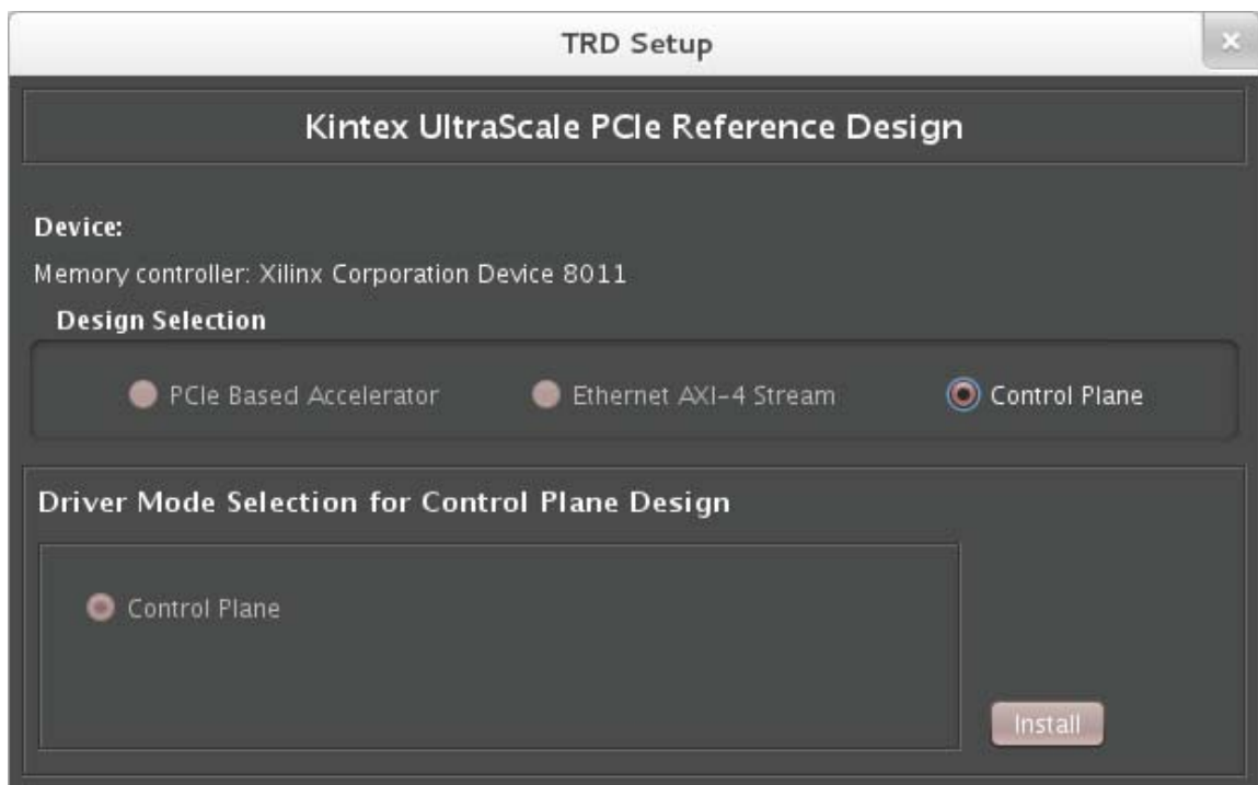
Figure 3-8: TRD Setup Screen with a PCIe Device Detected
