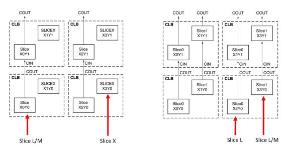
Figure 1 – Spartan-6 and 7 Series CLB Structure
