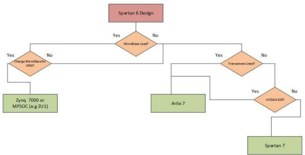
Figure 5 – Device Selection Spartan-6 to 7 Series Flow Chart
