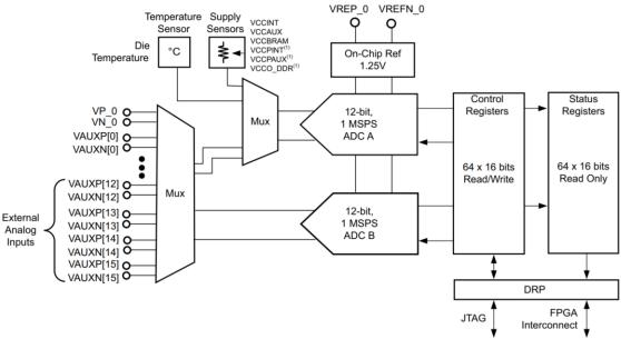
Figure 4 – XADC Structure 7 Series
