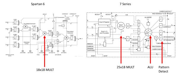
Figure 3 – Spartan-6 DSP48A1 and 7 Series DSP48E1 Structures
