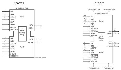
Figure 2 – Spartan-6 and 7 Series Block RAM Blocks
