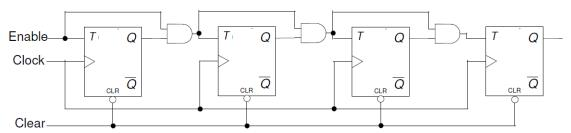
2-1. Design a 8-bit counter using T flip-flops, extending the above structure to 8-bits. Your design needs to be hierarchical, using a T flip-flop in behavioral modeling, and rest either in dataflow or gate-level modeling. Develop a testbench and validate the design. Assign Clock input, Clear\_n, Enable, and Q. Implement the design and verify the functionality in hardware.
