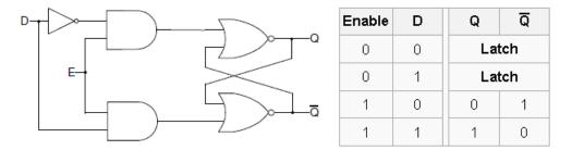
D-latches can be modeled in behavioral modeling as shown below.
