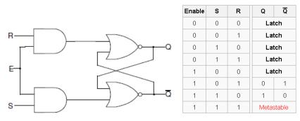
1-2. Design a gated SR latch (shown in the figure above) using dataflow modeling. Synthesize the design and view the schematic of the Open Synthesized Design. Develop a testbench to test (generate input as shown below) and validate the design. Simulate the design. Assign S input to SW0, R input to SW1, and Enable input to SW2. Assign Q to LED0 and Qbar to LED1. Implement the design and verify the functionality in the hardware.
