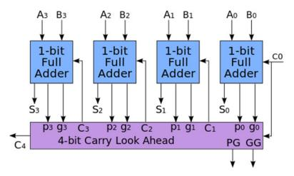
Where  $P_i = A_i + B_i$  and  $G_i = A_iB_i$ . Within Carry Look Ahead unit,  $C_{i+1} = G_i + P_iC_i$ . The speed-up is achieved through the fact that  $C_i$  being generated at the same time irrespective of  $i^{th}$  position.
