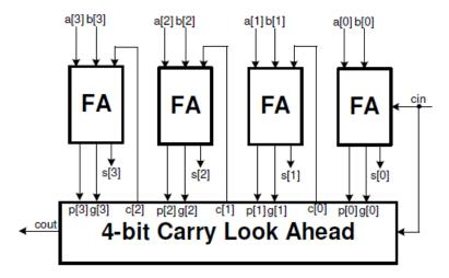
Where  $P_i = A_i + B_i$  and  $G_i = A_iB_i$ . Within Carry Look Ahead unit,  $C_{i+1} = G_i + P_iC_i$ . The speed-up is achieved through the fact that  $C_i$  being generated at the same time irrespective of i<sup>th</sup> position.
