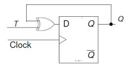
2-2. Modify the 8-bit counter using D flip-flops. The design should be hierarchical, defining D flip-flop in behavioral modeling, creating T flip-flop from the D flip-flop, implementing additional functionality using dataflow modeling. Assign Clock input to SW15, Clear\_n to SW0, Enable to SW1, and Q to LED7-LED0. Implement the design and verify the functionality in hardware.
