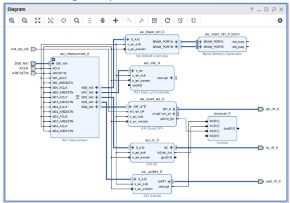
At this point, you have connected the interrupt signals to the Concat block, and there is a remaining unconnected input pin. You could re-customize the block to include only the required number of inputs. For this tutorial, you will use the Constant block to tie the extra input down instead.
