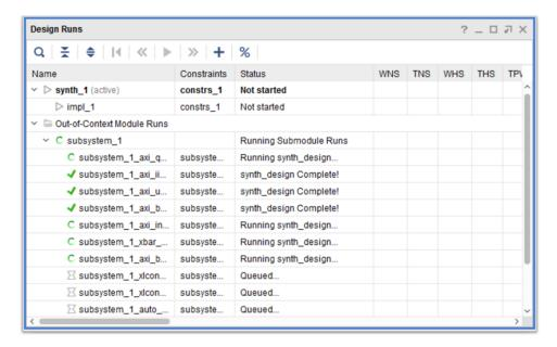
6. After the Out-of-context runs are finished, in the Sources window, right-click the top-level subsystem design, **subsystem\_1**, and select **Create HDL Wrapper**.
