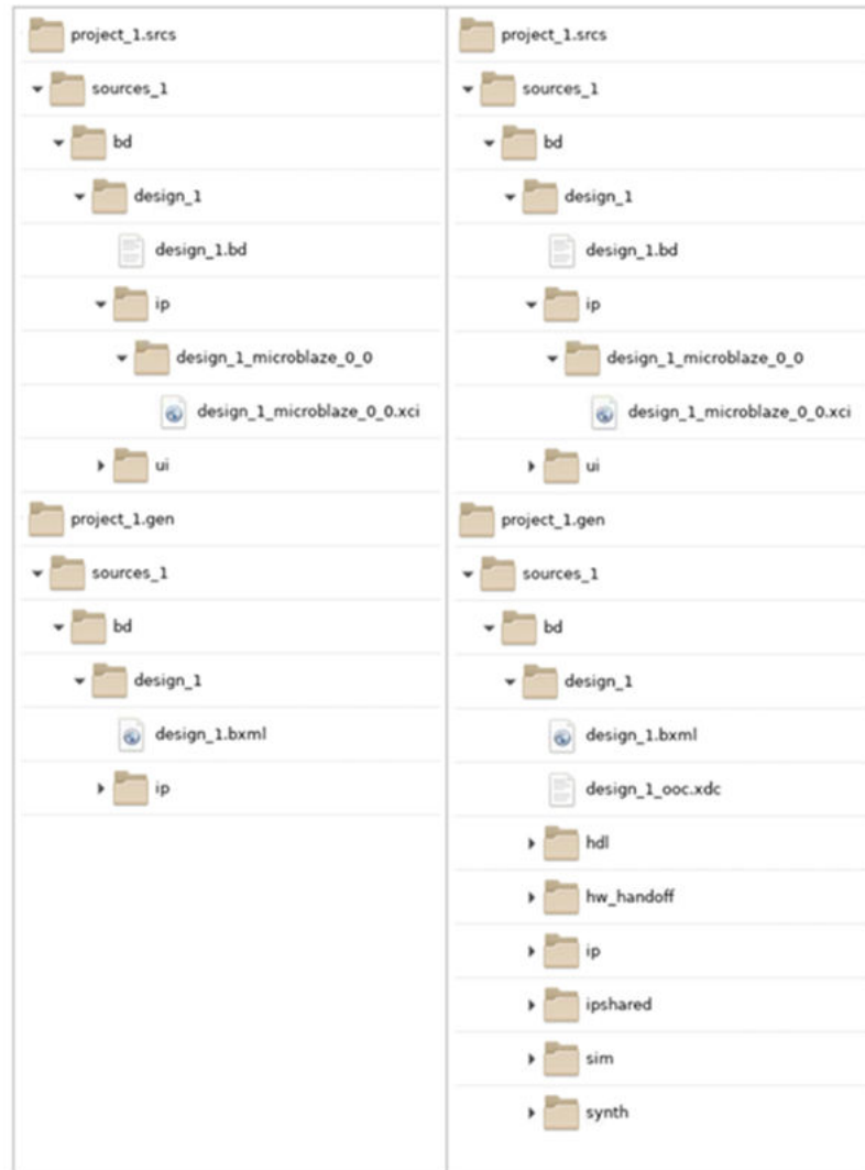
Figure 141: Directory Structure for Project IP and BD Files Before (Left) and After (Right) Generate Design
