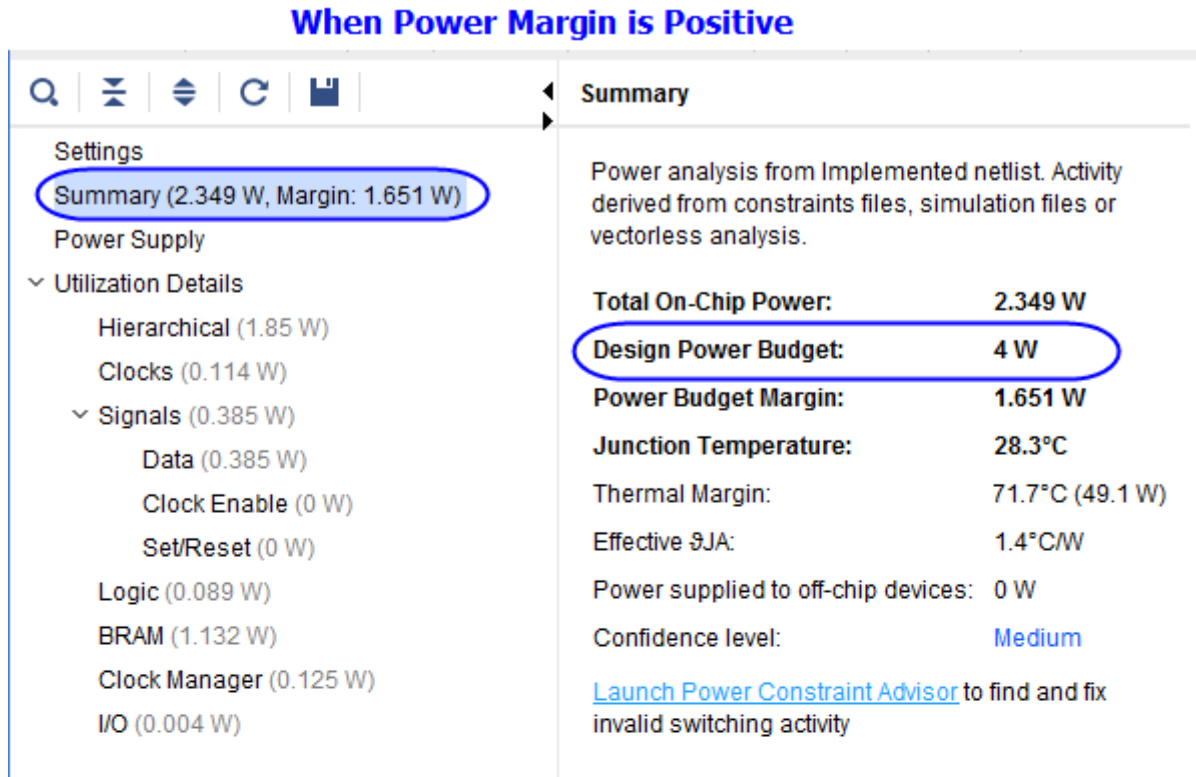
Figure 21: Power Report With Power Budget at Positive and Negative Margins
