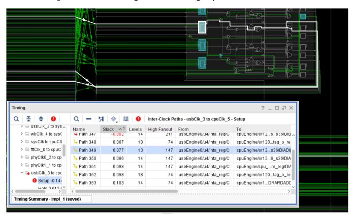
Figure 41: Cross-Probing Between Timing Report and Device Window
