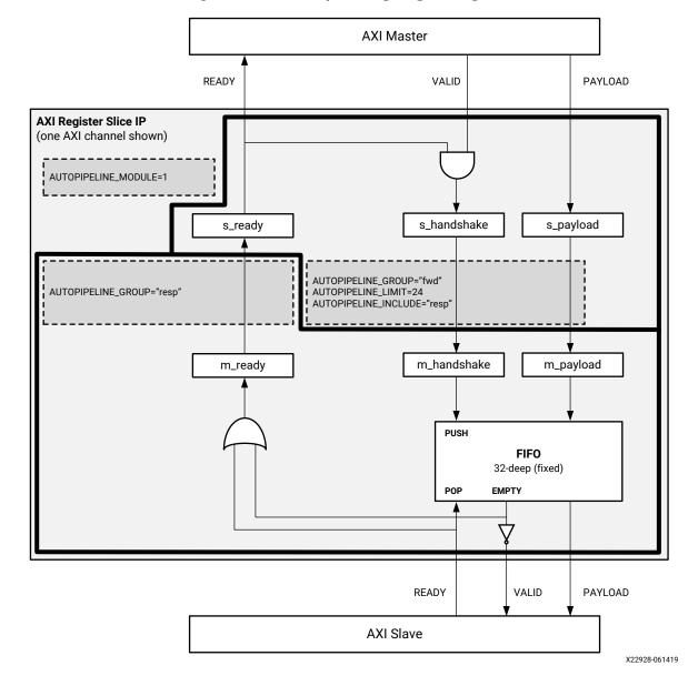
Figure 16: Auto-Pipelining Logic Diagram
