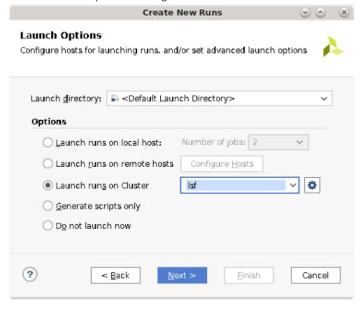
**Note:** The Launch runs on remote hosts and Launch runs on Cluster options shown in the previous figure are Linux-only. They are not visible on Windows machines.
