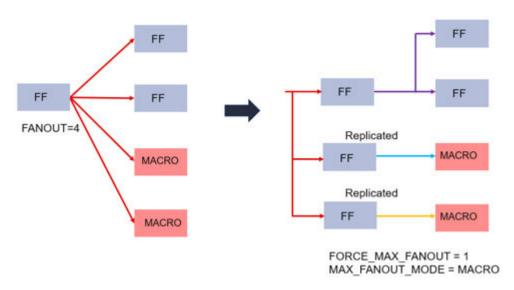
**Note:** This optimization happens early in the placer. In the later stages of the placer as the timing accuracy improves, both the replicated source and/or load registers may be moved to different clock regions or SLRs if the timing estimate improves.
