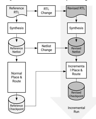
Figure 28: Incremental Compile Design Flow
