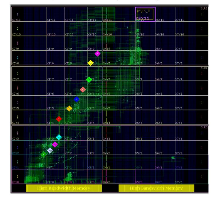
Figure 21: Device View of Auto-Pipeline Inserted Registers
