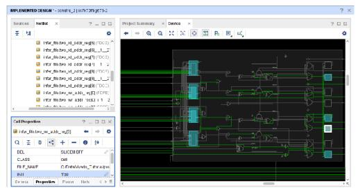
These properties can include everything from block RAM INITs to the clock modifying properties on MMCMs. There is also a special dialog box to set or modify INIT on LUT objects. This dialog box allows you to specify the LUT equation and have the tools determine the appropriate INIT.
