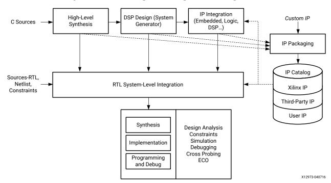
Figure 1: Vivado Design Suite High-Level Design Flow
