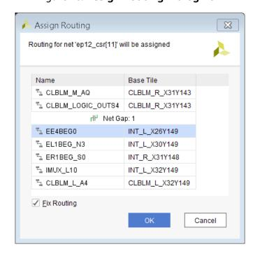
Figure 46: Assign Routing Dialog Box
