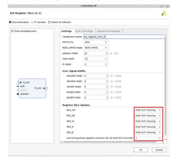
Figure 14: Example AXI Register Slice IP Settings to Enable Auto-Pipelining Feature
