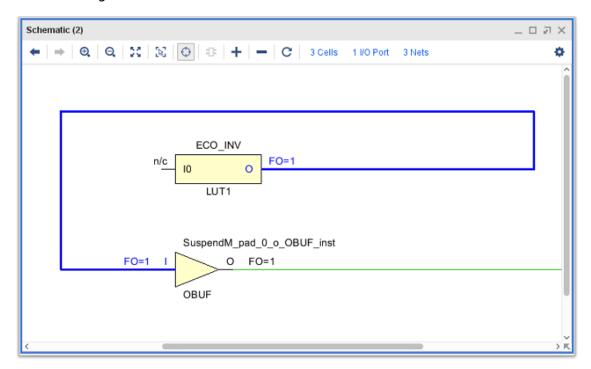
Figure 51: Schematic After Connection of LUT1 to an OBUF
