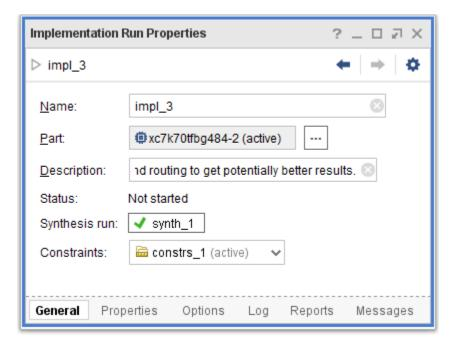
Figure 4: Implementation Run Properties Window
