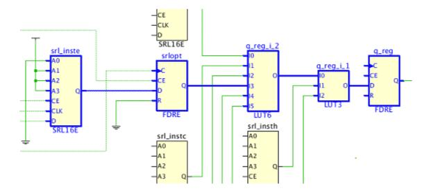
Figure 23: Critical Path after Shift Register Optimization
