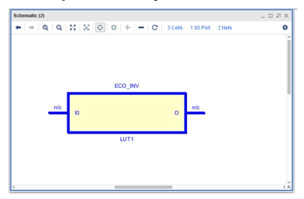
Figure 50: Cell Created Using LUT1 as a Reference Cell
