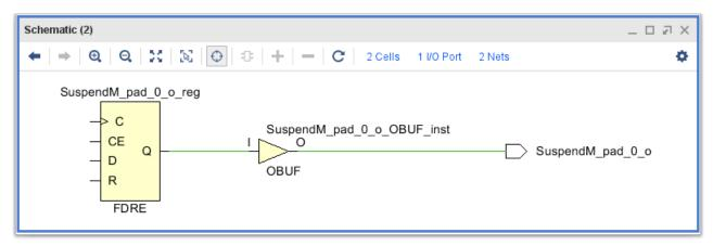
The following Tcl commands show how to add an inverter between the output of the FDRE and the OBUF:
