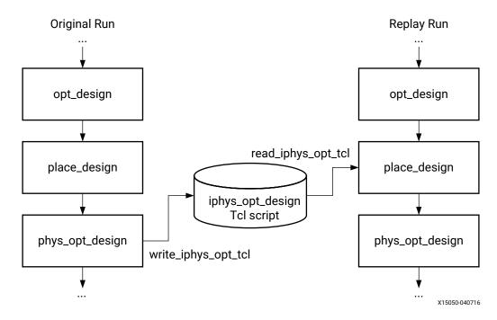
Figure 26: Design Flow Involving Retrofit
