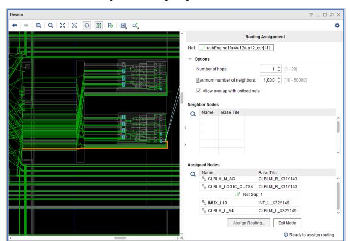
Figure 44: Routing Assignment Window
