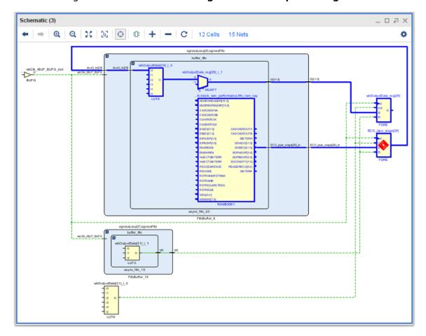
Figure 57: Schematic Showing Addition of Pipeline Register
