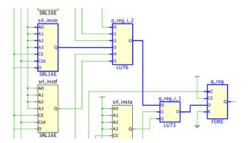
Figure 22: Critical Path Starting at Shift Register srl\_inste
