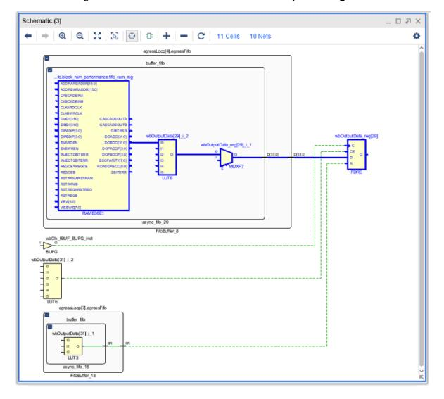
Figure 56: Schematic Prior to Addition of Pipeline Register
