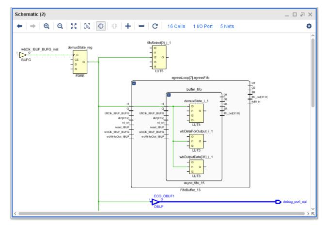
Figure 55: Schematic after Adding/Routing a Debug Port
