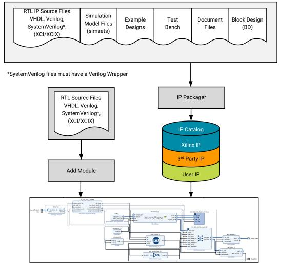
Figure 1: IP Packaging and Usage Flow
