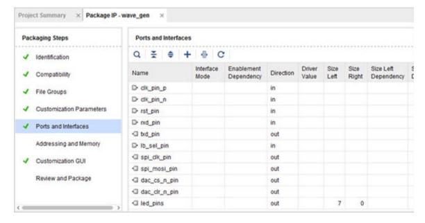
Figure 15: Package IP Window: Ports and Interfaces Page
