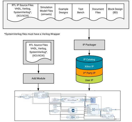
Figure 20: IP Packaging and Usage Flow
