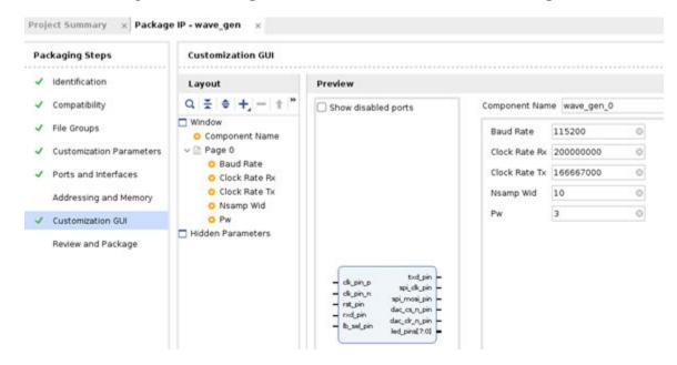
Figure 17: Package IP Window: Customization GUI Page
