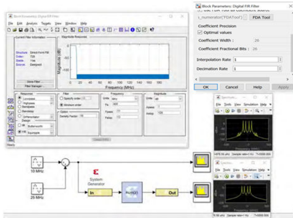
Figure 299: Digital FIR Filter Example
