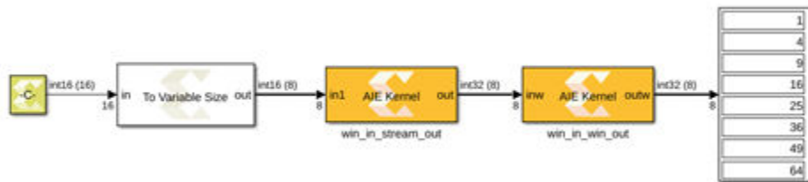
Figure 234: AIE Kernel: Window Input/Stream Output
