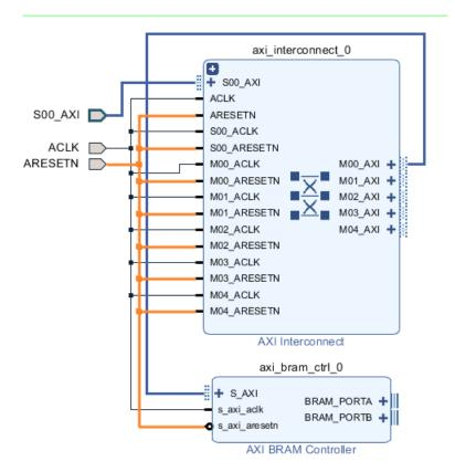
7. Using the same steps, connect the remaining slave IP cores in the design to the AXI Interconnect.
