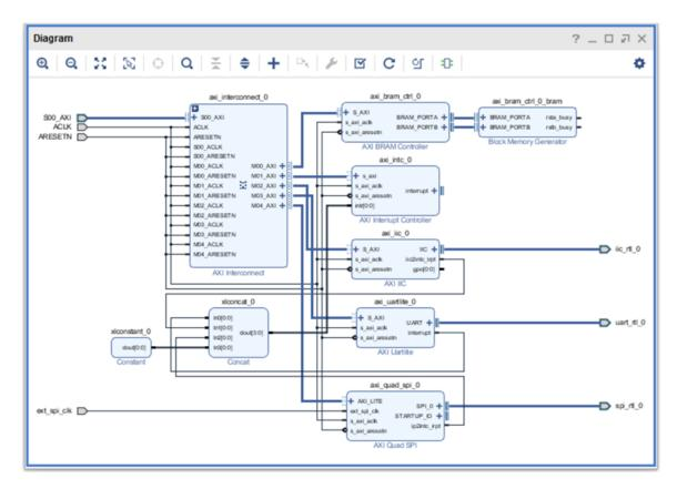
**Note:** The 1-bit bus width of the interrupt signal on the Interrupt Controller block does not match the 4-bit signal width from the Concat block. The Vivado tools correct this automatically during design validation.
