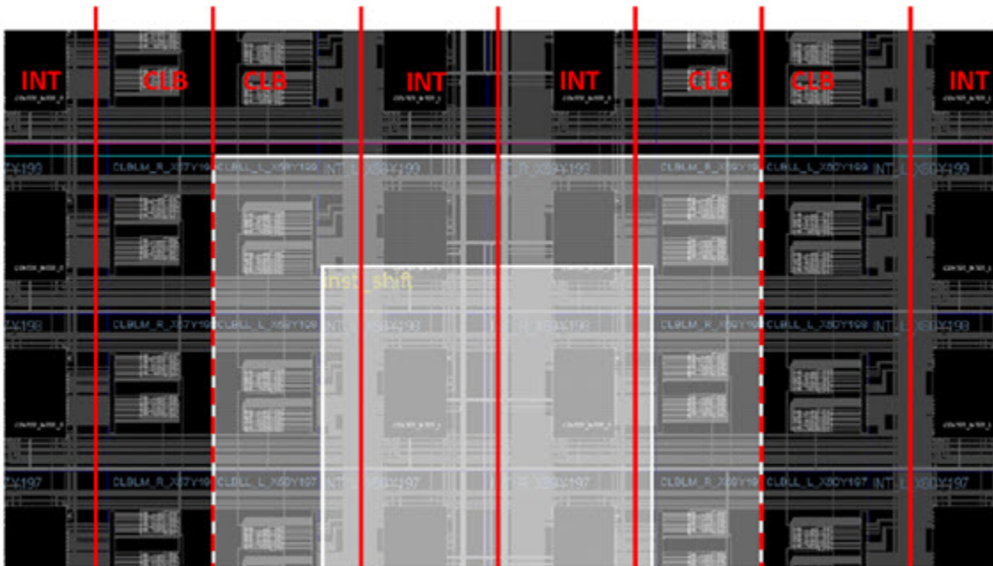
Figure 57: Optimal - Reconfigurable Partition Pblock Splitting CLB-CLB on Both Left and Right Edges
