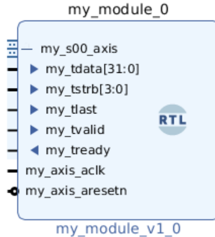
Figure 19: RTL Module with Custom AXI4-Stream Interface
