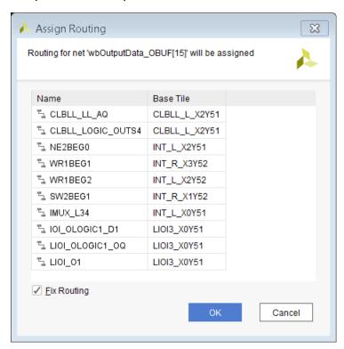
You routed the wbOutputData\_OBUF[14] and wbOutputData\_OBUF[15] nets with the detour to add the needed delay. You can now run the Report Datasheet command again to examine the timing for these nets with respect to the lower order bits of the bus.
