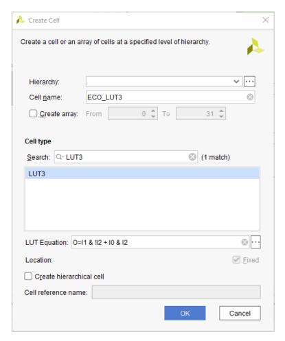
Because you copied the LUT equation from cell  $count_out[3]_{i=1}$ , the nets must be hooked up in the same order, with the following connections:
