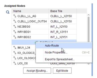
The Vivado router fills in the last small bit of the gap. With the route path fully defined, you can assign the routing to commit the changes to the design.
