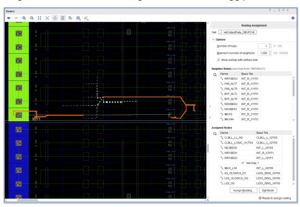
12. Under the Assigned Nodes section of the Routing Assignment window, right-click the **Net Gap**, and select **Auto-Route**, as shown in the following figure.
