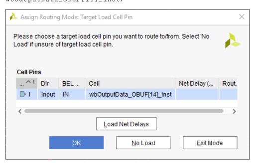
7. Select the load cell pin wbOutputData\_OBUF[14]\_inst/I, and click OK.
