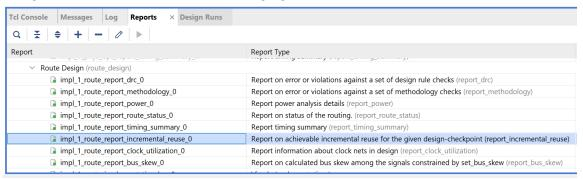
So far, you have modified the generation of the readEgressFifo so that the signal is zero when the error signal is non-zero. This is a small change to the design so you would expect the reuse to be high. Now examine the Incremental Reuse Report to confirm this is the case.
