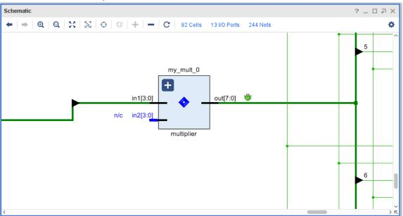
The Tcl Console reproduces the disconnect\_net command that you just executed in the ECO Navigator. This is useful if you want to replay your ECO changes later by opening the original checkpoint and sourcing a Tcl script with the ECO commands.
