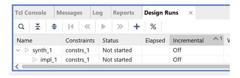
This column shows how the incremental flow was used. The information is also available in the messages in the Vivado log file.
