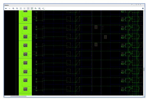
Having routed all the upper bit nets, wbOutputData\_OBUF[31:14], with the detour needed for added delay, you can now re-examine the timing of output bus.
