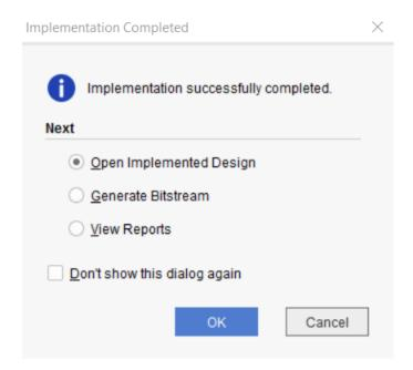
In a project-based design, the Vivado Design Suite saves intermediate implementation results as design checkpoints in the implementation runs directory. You will use the final checkpoint as the reference to the incremental compile flow.
