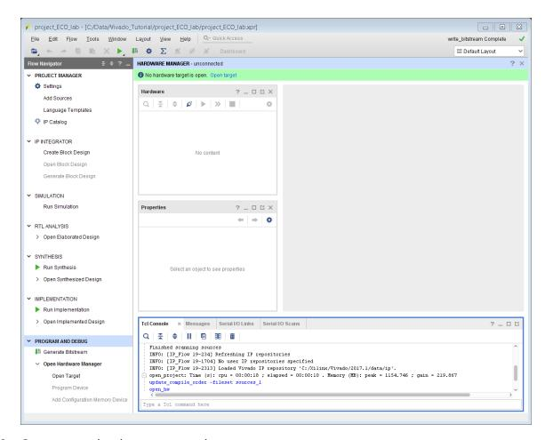
2. Connect to a hardware target using hw\_server.
