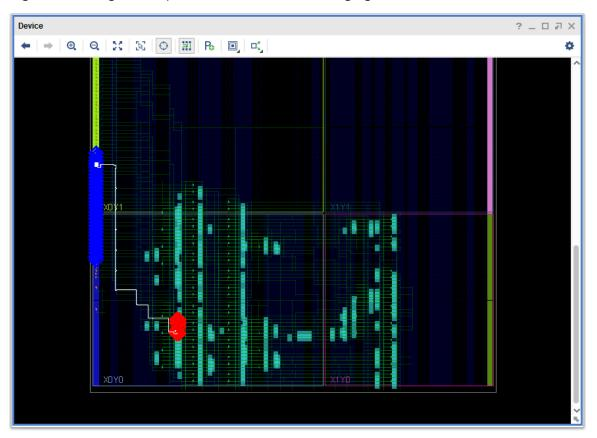
The outputs marked in blue are spread out along two banks on the left side starting with wbOutputData[0] (on the bottom) and ending with wbOutputData[31] (at the top), while the output registers marked in red are clustered close together on the right.
