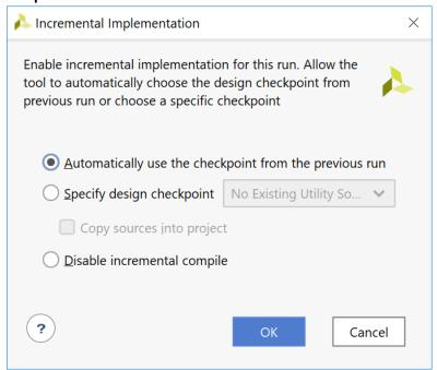
This dialog box can be opened from many places inside the Vivado IDE. These include the Implementation Run Options window and the Project Summary. The same functionality can also be built into scripts via Tcl commands.
