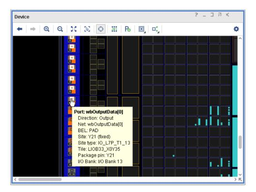
The bottom ports are the lowest bits of the output bus, starting with wbOutputData[0].
