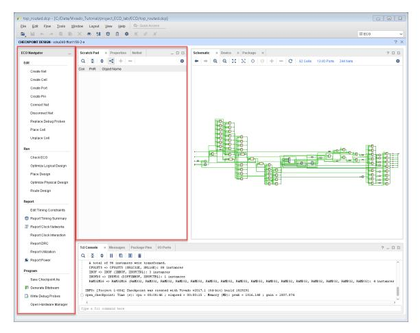
To illustrate the capabilities of the ECO flow, you next change the functionality of the multiplier from a square of count [3:0] to a multiply by two.
