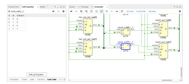
This command selects the LUT2 that drives the  $count_out_reg[7]$  register, which drives LED 7 on the KCU105 board. The only inputs are  $tog_state_reg$  for pin I0 and  $mul_out_pre_reg[7]$  for pin I1. You need to replace the LUT2 with a 3-input LUT and connect the output of counter register  $divClk_reg[24]$  to the additional input pin.
