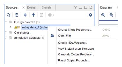
The Generate Output Product dialog box opens, as shown in the figure below, to regenerate the various output products associated with the subsystem design.
