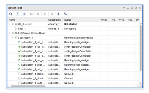
6. After the Out-of-context runs are finished, in the Sources window, right-click the top-level subsystem design, **subsystem\_1**, and select **Create HDL Wrapper**.
