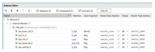
4. Change the size of the address segments for the AXI BRAM Controller core.
