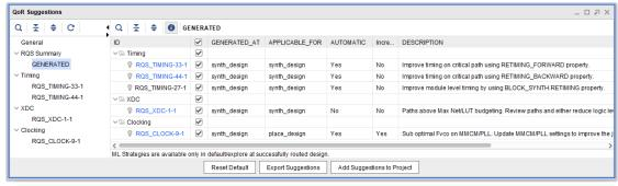
The GENERATED section provides a list of all the suggestions that have just been generated at this stage of the current run. Each suggestion has a description that details the reason for the suggestion. Additionally, for each suggestion the following information is provided.
