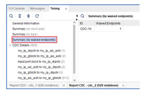
The detailed section for the  $my_{ip_glblclk}$  to  $my_{ip_axi_aclk}$  CDC shows that the Critical CDC-10 was replaced with an Info CDC-3.
