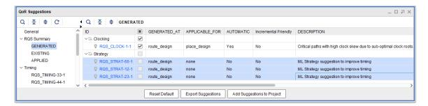
9. Select RQS\_STRAT-66-1. Here you can see the details of the strategy being recommended. It is possible to see the details of the strategy suggested. It would be possible manually set these up as shown but in order to automate the process more easily, the recommended flow is to read an RQS file containing strategies, and set the directive to RQS on the implementation commands.
