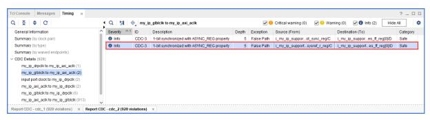
7. Select the new CDC-3 row, and click the Schematic toolbar button in Double-click the Q pin of the output register to expand the schematic to match what is shown in the following figure.
