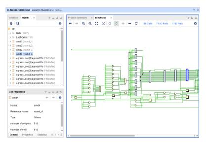
Figure 47: Elaborated Design in the RTL Schematic Window
