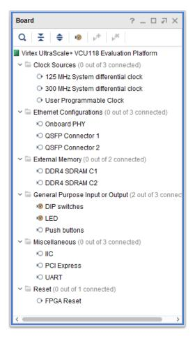
Figure 12: Board Window in Vivado IP Integrator
