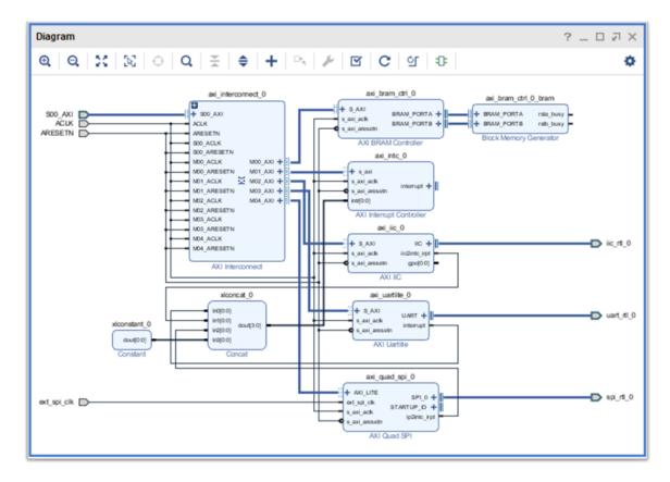
**Note:** The 1-bit bus width of the interrupt signal on the Interrupt Controller block does not match the 4-bit signal width from the Concat block. The Vivado tools correct this automatically during design validation.
