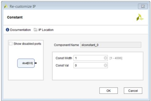
The fourth input of the Concat block is no longer floating. Now you can connect the concatenated interrupt signals from the Concat block to the Interrupt Controller.
