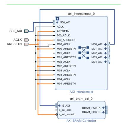
Using the same steps, connect the remaining slave IP cores in the design to the AXI Interconnect.
