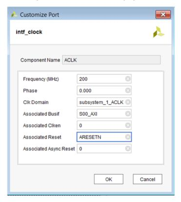
Now you can connect the AXI clock and reset nets to the remaining master and slave clocks and resets of the AXI Interconnect.
