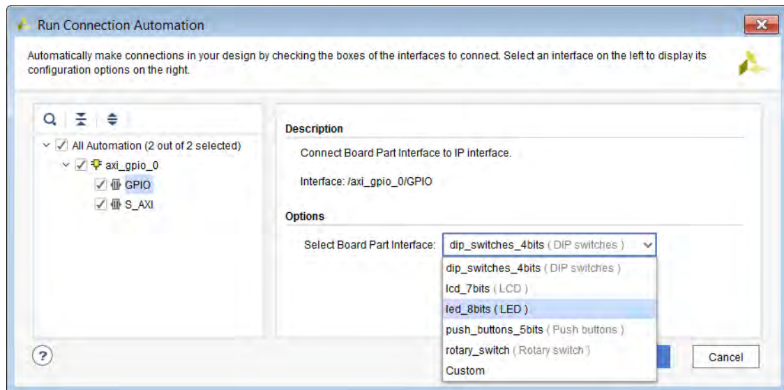
Figure 17: Using Connection Automation to Show Potential Connections
