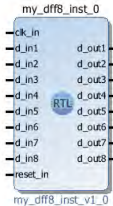
Figure 4: Modules Referenced from an RTL Source file
