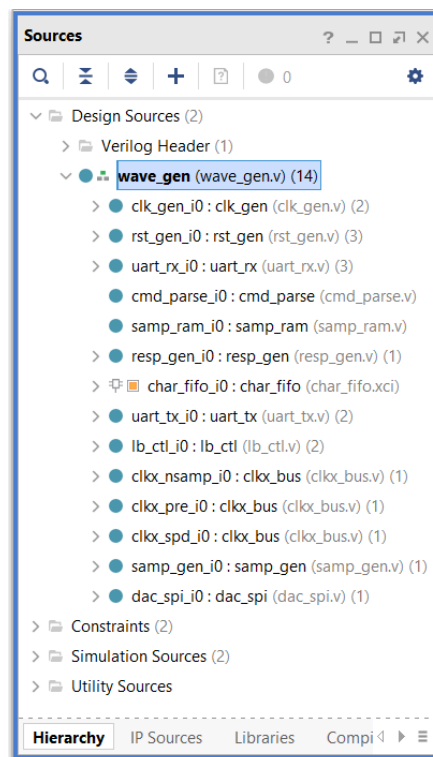
Figure 13: IP Integrated into the Design
