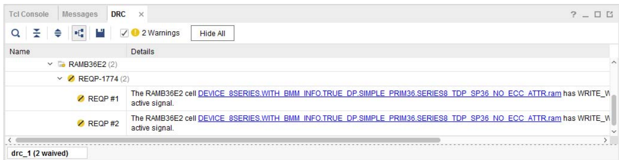
Figure 4-8: Waived DRC Violations
