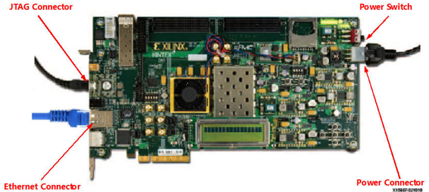
Figure 121: KC705 Board Ethernet Connections
