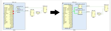
Following is an example of a clock uncertainty reduction for clock domain crossing (CDC) paths between a 150 MHz clock and a 300 MHz clock:
