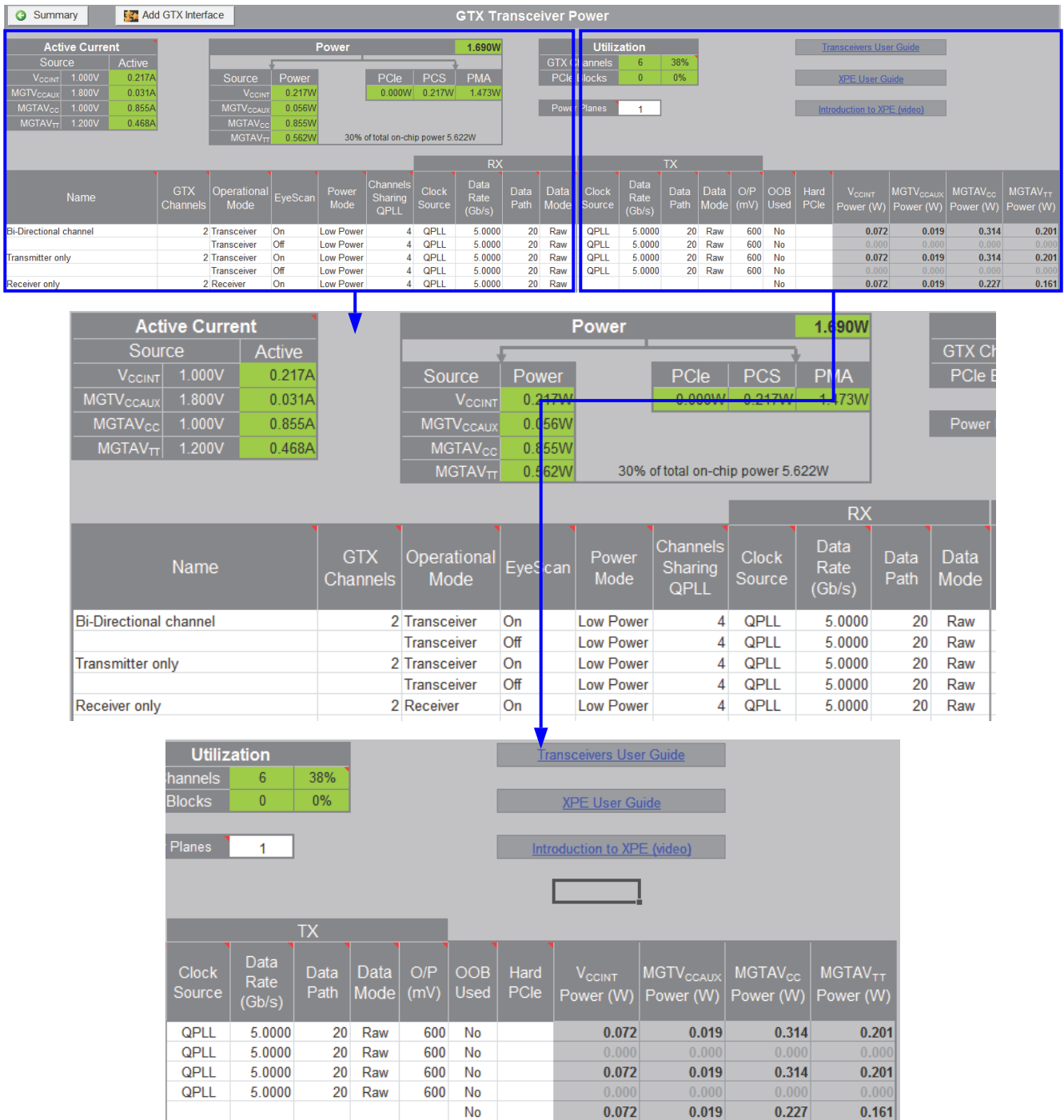
Figure 3-12: GT Power Sheet (Kintex-7 Devices) Illustrating Data Rate and Power Estimates
