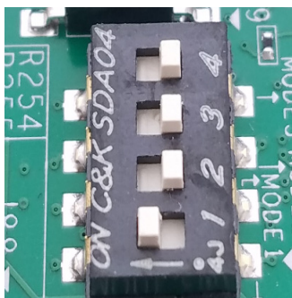
Figure 5-7: SW6 Switch Settings for SD Boot Mode
