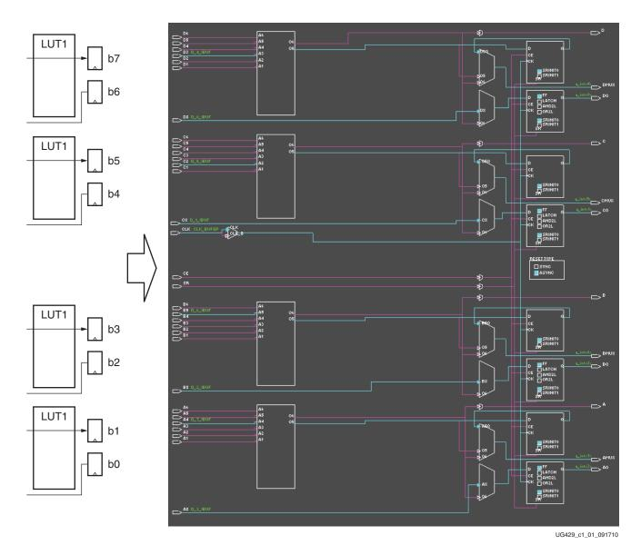
Figure 1-1: FPGA Editor Representation of a Route-Thru
