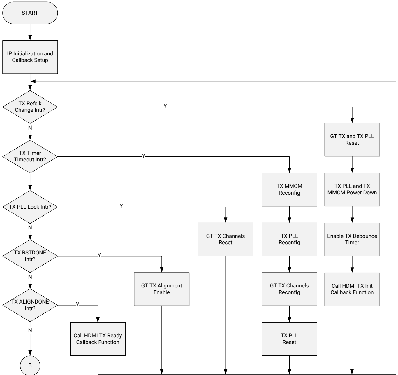
Figure 18: HDMI TX Program Flow
