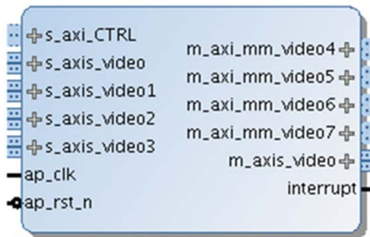
Figure 2-1: Video Mixer I/O Diagram
