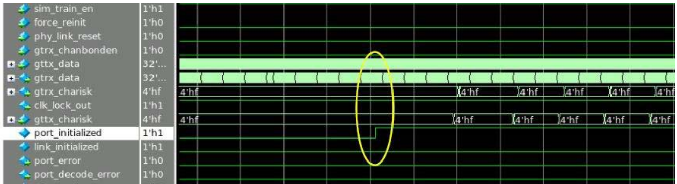
Figure C-3: port_initialized and link_initialized Signals
