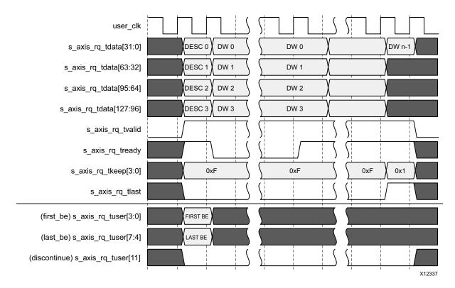
Figure 3-48: Memory Write Transaction on the Requester Request Interface (Dword-Aligned Mode, 128-Bit Interface)
