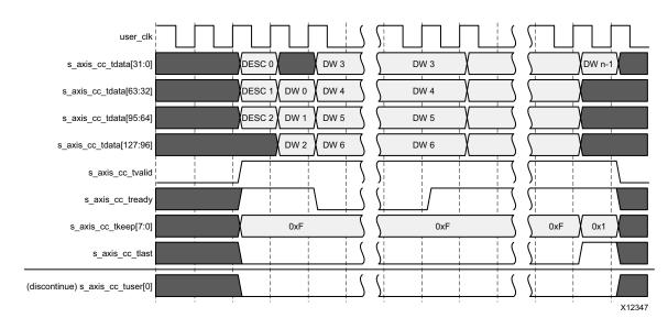
Figure 3-38: Transfer of a Normal Completion on the Completer Completion Interface (Address-Aligned Mode, 128-Bit Interface)
