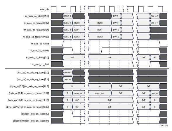
Figure 3-27: Memory Write Transaction on the Completer Request Interface (Address-Aligned Mode, 128-Bit Interface)
