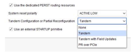
Figure 3-4: Tandem Configuration or Partial Reconfiguration Option
