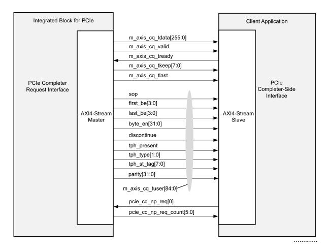
Figure 3-18: Completer Request Interface Signals
