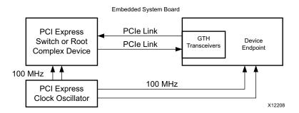
Figure 3-15: Embedded System Using 100 MHz Reference Clock
