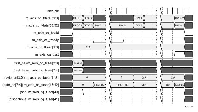
Figure 3-26: Memory Write Transaction on the Completer Request Interface (Address-Aligned Mode, 64-Bit Interface)
