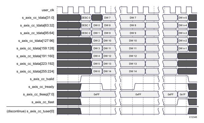
Figure 3-39: Transfer of a Normal Completion on the Completer Completion Interface (Address-Aligned Mode, 256-Bit Interface)
