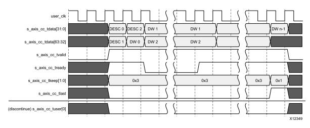
Figure 3-34: Transfer of a Normal Completion on the Completer Completion Interface (Dword-Aligned Mode, 64-Bit Interface)
