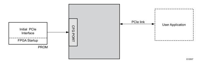
Figure 3-8: Tandem PCIe Bitstream Load Steps
