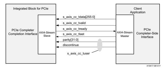
Figure 3-32: Completer Completion Interface Signals
