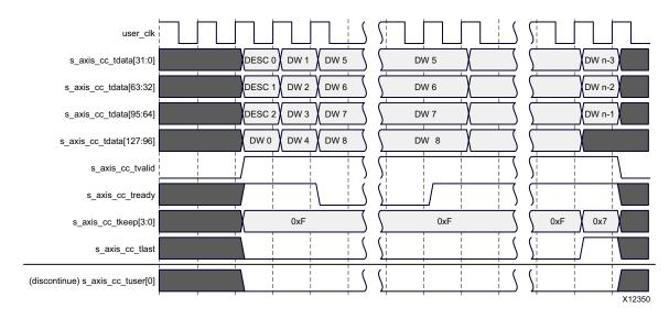
Figure 3-35: Transfer of a Normal Completion on the Completer Completion Interface (Dword-Aligned Mode, 128-Bit Interface)
