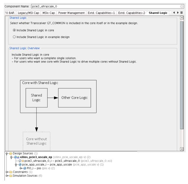
Figure 3-1: Shared Logic in the Core
