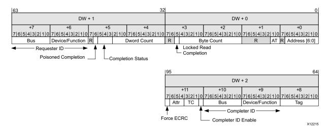
Figure 3-33: Completer Completion Descriptor Format
