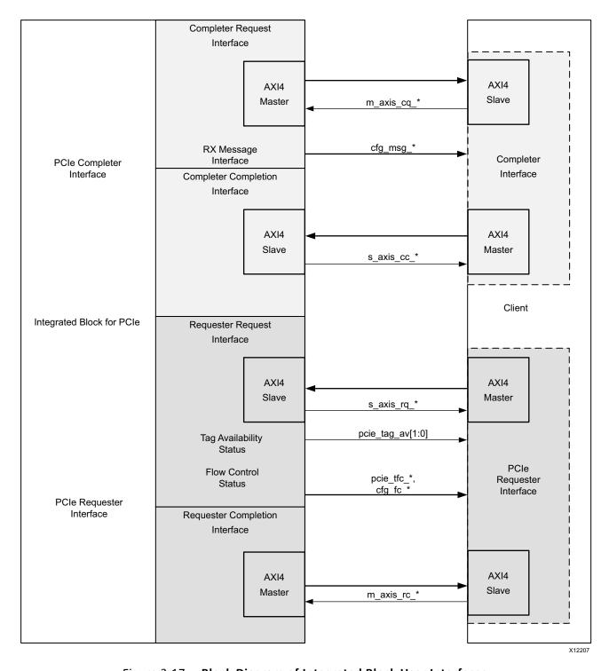
Figure 3-17: Block Diagram of Integrated Block User Interfaces
