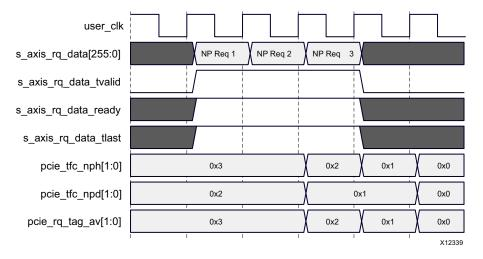
Figure 3-56: Credit and Tag Availability Signals on the Requester Request Interface (256-Bit Interface)
