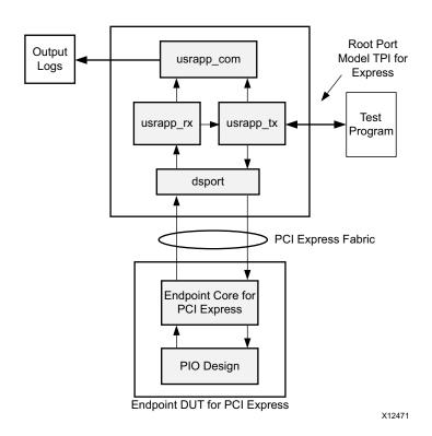
Figure 5-1: Simulation Example Design Block Diagram
