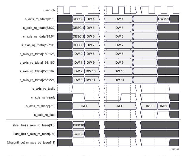
Figure 3-49: Memory Write Transaction on the Requester Request Interface (Dword-Aligned Mode, 256-Bit Interface)
