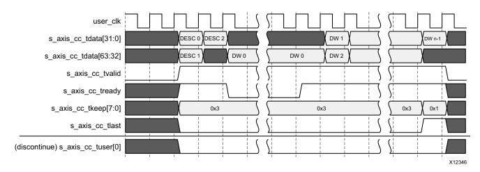
Figure 3-37: Transfer of a Normal Completion on the Completer Completion Interface (Address-Aligned Mode, 64-Bit Interface)
