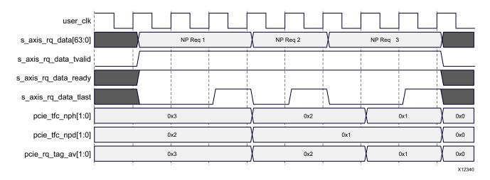
Figure 3-58: Credit and Tag Availability Signals on the Requester Request Interface (64-Bit Interface)
