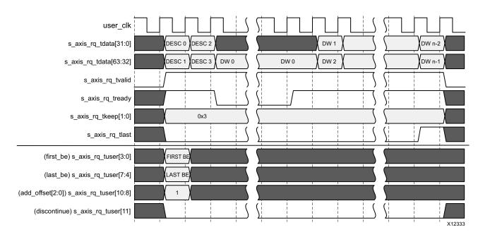
Figure 3-50: Memory Write Transaction on the Requester Request Interface (Address-Aligned Mode, 64-Bit Interface)
