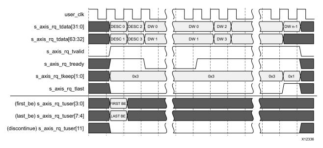
Figure 3-47: Memory Write Transaction on the Requester Request Interface (Dword-Aligned Mode, 64-Bit Interface)
