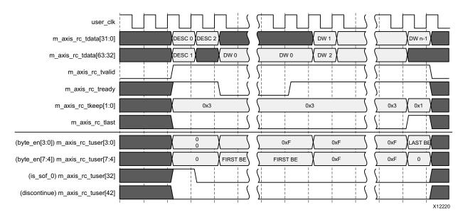
Figure 3-67: Transfer of a Completion with Data on the Requester Completion Interface (Address-Aligned Mode, 64-Bit Interface)
