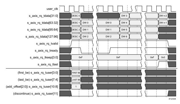
Figure 3-51: Memory Write Transaction on the Requester Request Interface (Address-Aligned Mode, 128-Bit Interface)
