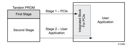
Figure 3-5: Tandem PROM Bitstream Load Steps
