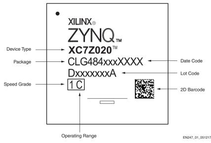
Figure 1: Example Device Top Mark
