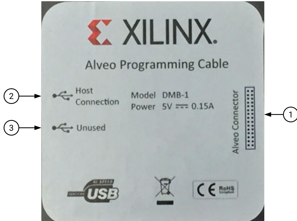
Figure 1: Alveo Programming Module Interface Locations
