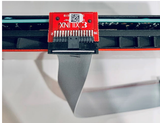
Figure 6: U25 Adapter Connected to the Alveo U25 Card
