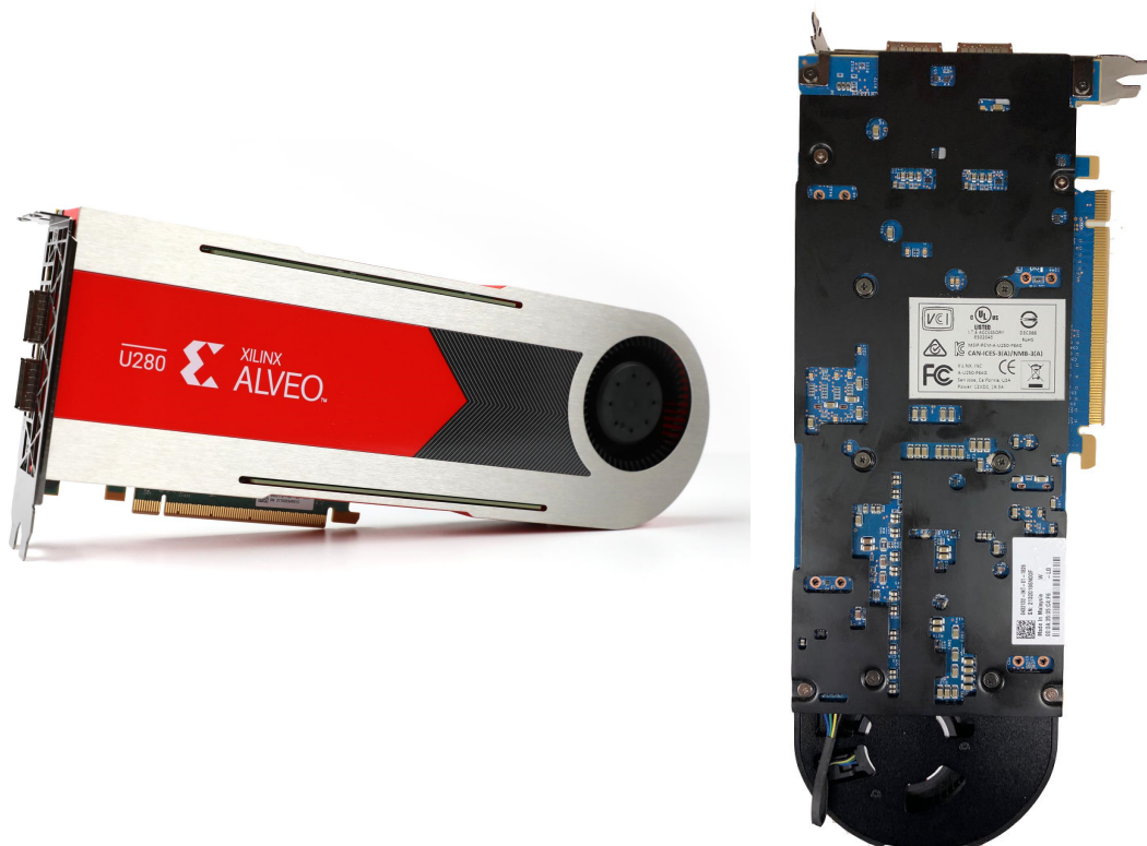
Figure 3: Passive Cooled Card Configuration
