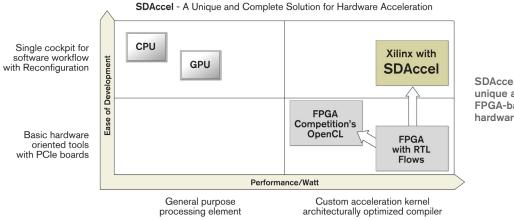
SDAccel represents a unique and complete FPGA-based solution for hardware acceleration
