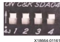
Figure 22: MODE[3:0] DIP Switch Setting (ON ON ON ON)
