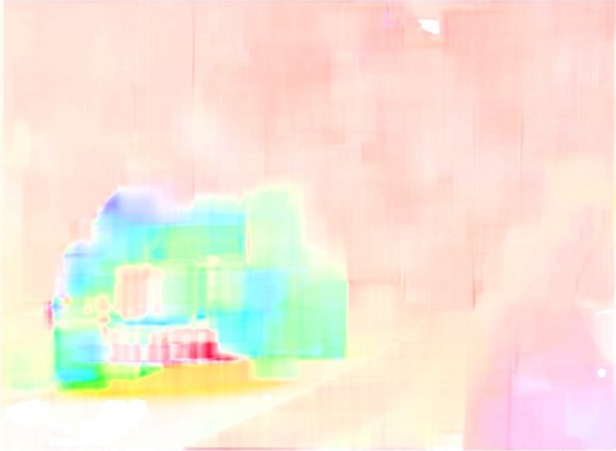
Figure 7: Motion Vectors Generated via a 43x43 Integration Window
