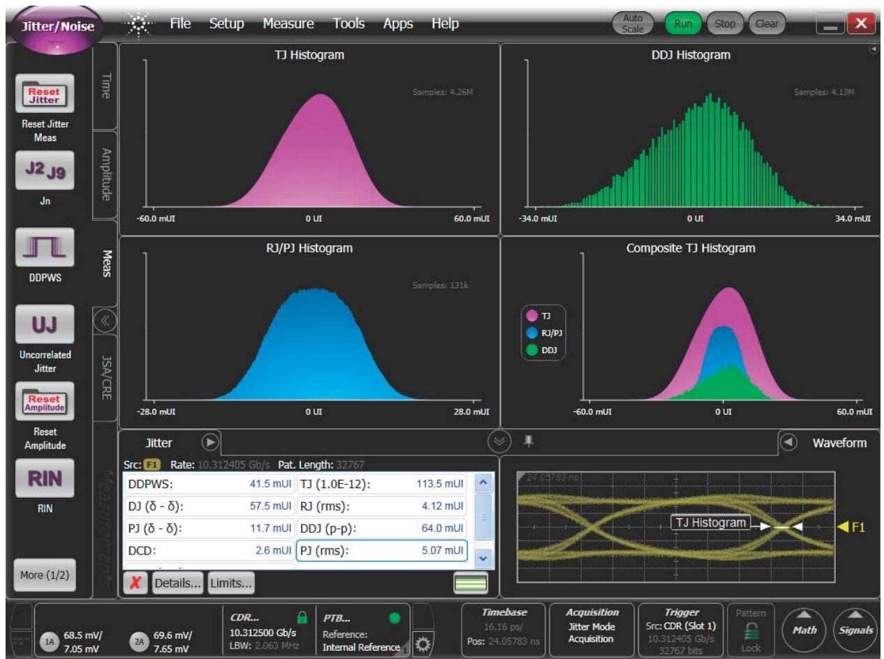
Figure 11: 10.3125 Gb/s Output Jitter Decomposition
