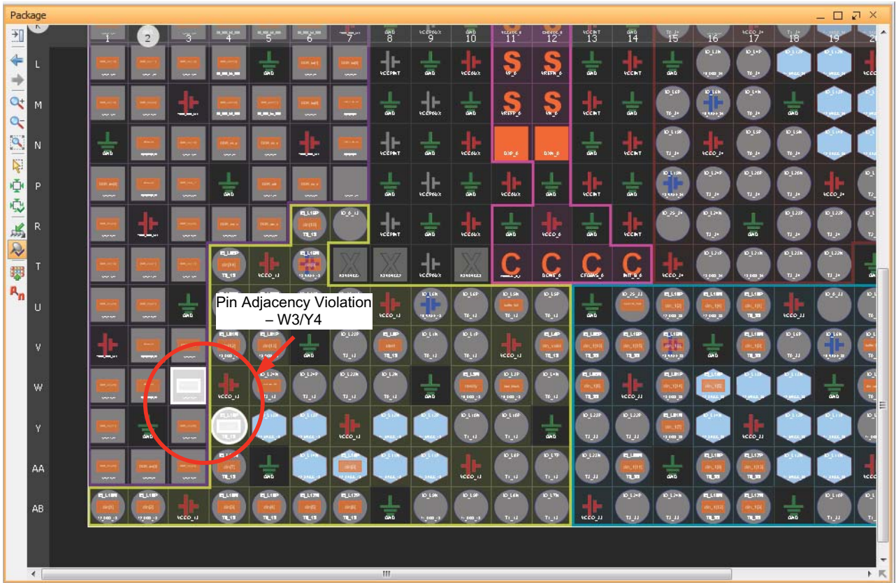
Figure 11: Pin Adjacency Violations Highlighted in Package Window
