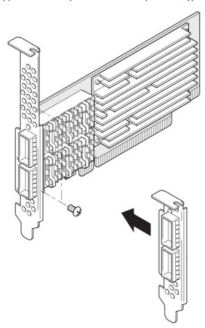
An optional 1PPS bracket and cable assembly, Solarflare part number SOLR-PPS-DP40G, is available for Solarflare dual-port QSFP+ server adapters. For detailed fitting instructions, refer to the *Solarflare Server Adapter User Guide*.
