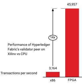
The Varium C1100 card is based on Xilinx UltraScale+. Estimated results are based on Intel Xeon Silver 4114 vs Xilinx UltraScale+ transactions / sec.
