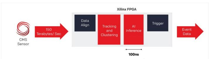
Figure 2: Compared to alternative devices such as GPUs and ASICs, FPGAs are the only viable choice for the event trigger processing because they provide extremely low latency. While the large numerical processing capability of GPUs is attractive, these technologies are optimized for high throughput, not low latency.
