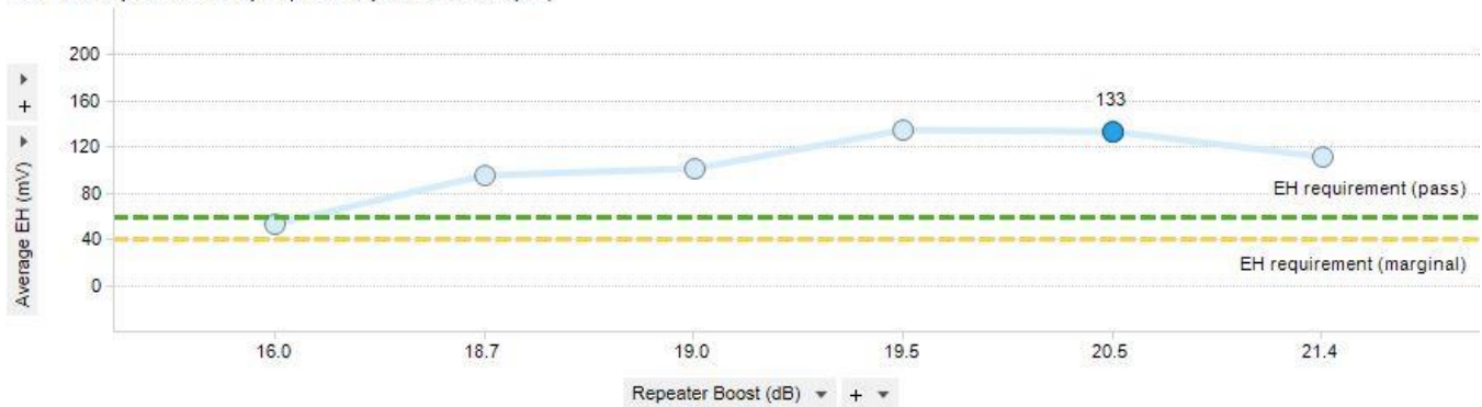
Figure 10: Rx Post-Equalized EH and EW vs. Repeater Boost
