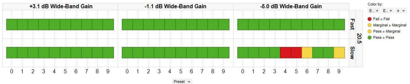
Figure 16: EH/EW Pass/Fail Result Across PVT and Different Wide-Band Gain Variations
