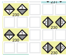
Figure 3. Ground pin wall separating TX and RX pins
