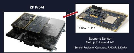
ZF ProAl is its modular hardware concept and open software architecture. This approach is unique compared to other systems on the market, which use a fixed combination of hardware and software architecture (which can limit functionality and add more cost)
